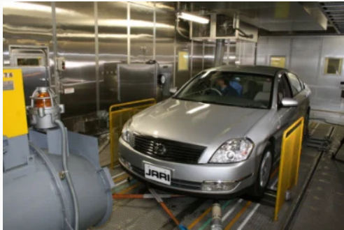
Figure 43: Example of Fuel Consumption Test
