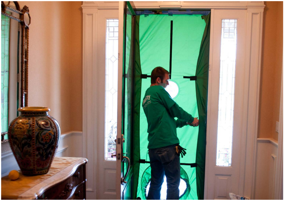
A home energy auditor conducts a blower door test to locate any unsealed cracks and openings.
