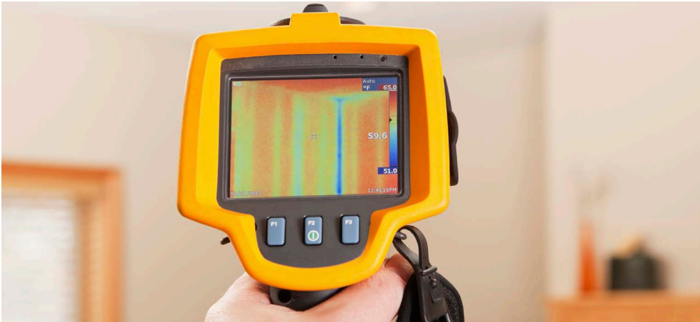
An infrared thermal imaging system shows a distinct cold (blue) area within the home's insulation.
